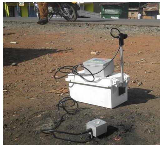
Photo 14: Vibration measurement meter (Nomis SuperMini® Seismograph)
