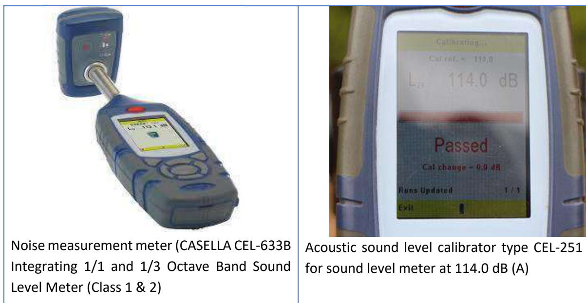
Figure 2-4: Calibration of equipment before undertaking measurements
