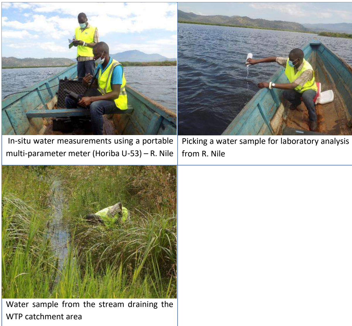
Figure 2-8: Taking in-situ water quality measurements and a water sample from River Nile and stream located downstream of the proposed WTP
